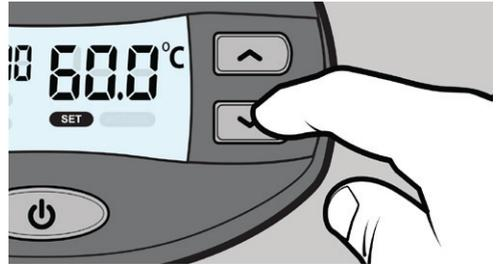
**NOTE:** To confirm SET temperature at any time, simply push the UP / DOWN arrow button – the display will briefly show the SET temperature before reverting back to ACTUAL temperature again.
