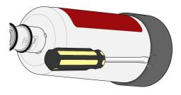
3. Align a flat screwdriver with the tab on the filter cap and gently push.
