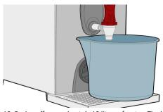
10. Drain –off approximately 10 litres of water. The boiler is now ready for use.
