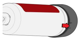
4. With one tab loosened, pull the filter cap off the old cartridge.
