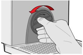
2. Grip Cartridge and rotate a quarter turn to the left and pull forward. CAUTION: A small amount will drain from the head and be directed to the front drip-tray as cartridge is removed.
