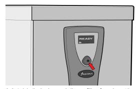
8. Switch boiler back on and allow to fill up for at least 15 minutes .
