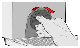
7. Insert new cartridge and turn until it locates. Install with a quarter turn to the right until cartridge comes to a complete stop (Inlet water will automatically turn on)
