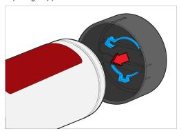
5. Align the shape on the inside of the filter cap (highlighted above) with the shape on the end of the new filter and push the two together until it clicks firmly in place.
