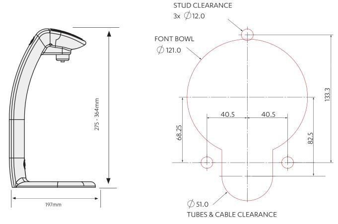
InstaTap mounting clearance - All dimensions in mm
