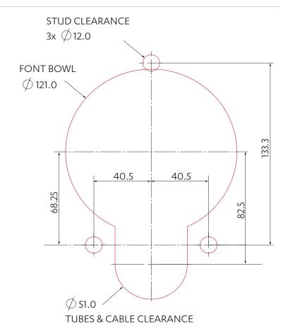
InstaTap mounting clearance - All dimensions in mm
